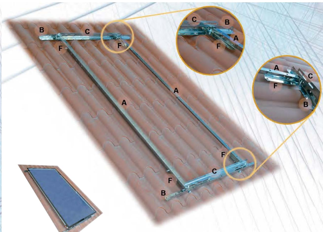
(EN) **NOTE:** Measures/Distances and inclination may be different, depending on the Assembly / Installation of the structure in place.
